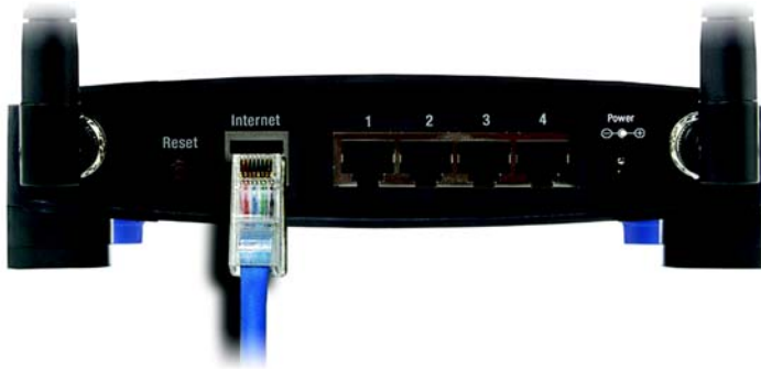
Figure 4-6: The Router with the Internet Connection is connected through the Internet Port
