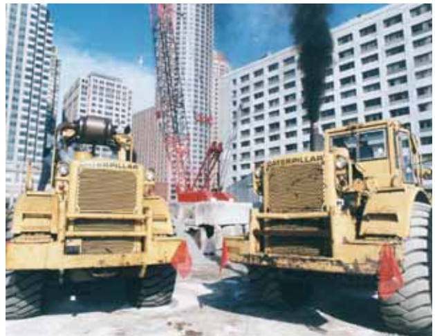
Retrofits are effective in reducing particle emissions from heavy equipment. The tractor on the left is retrofitted with a particle emissions control device.
